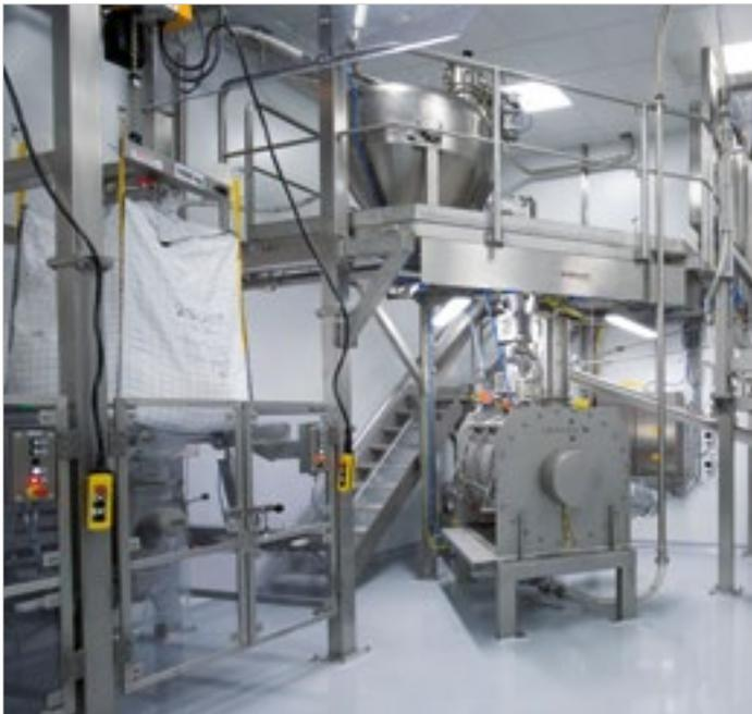
System example with mixing line, big bag station, storage vessel, liquid dosing and Lödige Ploughshare® Mixer FKM 1200 D
