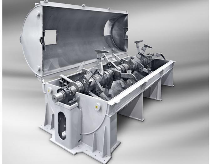
Optimal access to the inside of the drum
